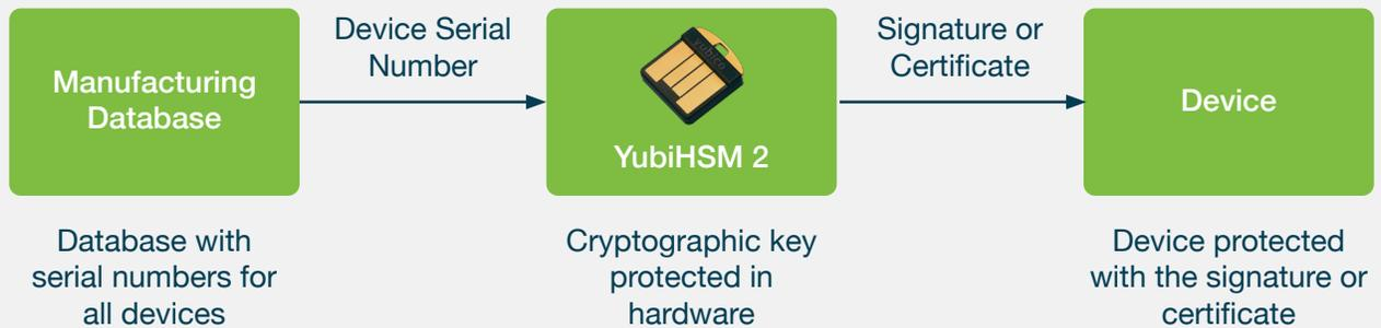
*Figure 1* (above) provides a high level process summary of the proposed solution to be implemented, as either a replacement or a brand new process in manufacturing plants and/or production lines, with the YubiHSM 2 at the core. The foremost point to highlight is that the cryptographic key used to sign and/or certify components is never exposed *outside* of the YubiHSM 2 hardware, thus ensuring a high level of security.
